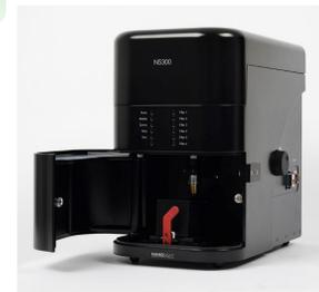
Nanoparticle Tracking Analysis (NTA) to characterize nanoparticle from 10-2000nm in solution. Each particle is individually but simultaneously analyzed by direct observations of diffusion. This particle-by-particle methodology produces high resolution results for particle size distribution and concentration while visual validation gives users extra confidence in the data.
