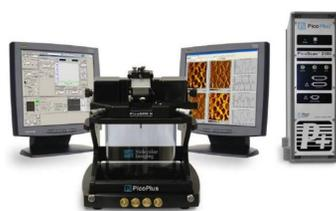
The NBTC second floor labs are equipped with an MI PicoPlus system specially designed for environmental and liquid imaging. The PicoPlus is well suited for in-vitro studies of both biological/soft materials as well as standard ambient imaging and it can be mounted on top of the TIRF fluorescent microscope for simultaneous fluorescent imaging of samples.
