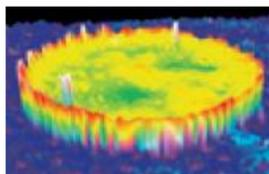
Ellipsometry is a well-known non-destructive optical method for determining film thickness and optical properties. Imaging Ellipsometry combines the power of ellipsometry with microscopy to allow spatial information on film thickness. Liquid measurement capability allows for in-vitro real-time measurements of thin film growth/corrosion.
